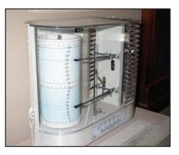
When properly calibrated, hygrothermographs are accurate
