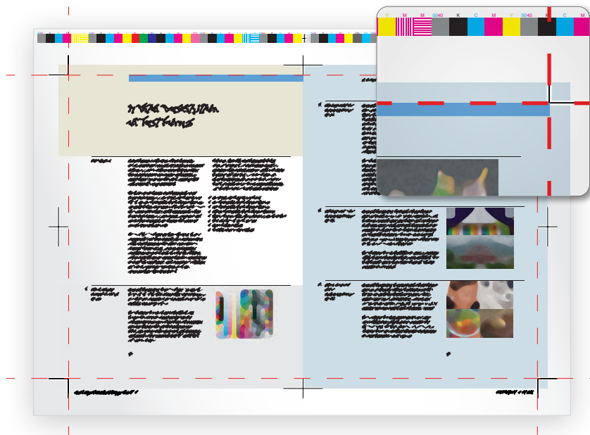
Figure 1. Sample offset lithography press sheet with a tail-edge color bar.
