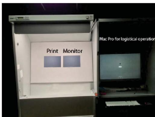
*Figure 1. Integrated soft proofing system*
