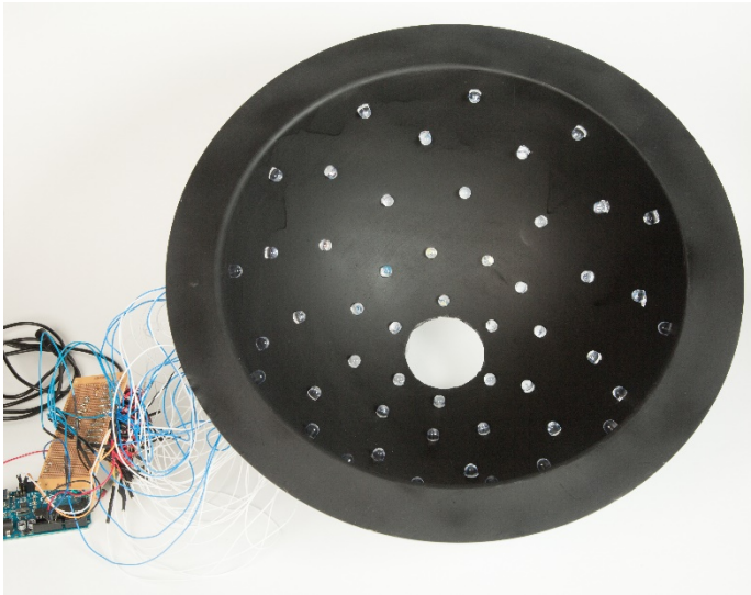
Figure 8. Inside of the large sphere showing the 50 LED lights. Each light is a 10 mm supper bright LED and can be independently controlled by the Aduino Uno microprocessor.
