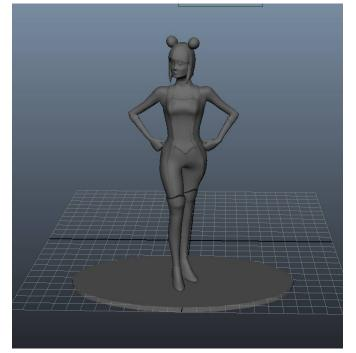
Our 3D Sara Lockhart model was created using AutoDesk Maya. We created it in two different pieces, the figure and the base. We then printed it on the MakerBot 3D printer.
