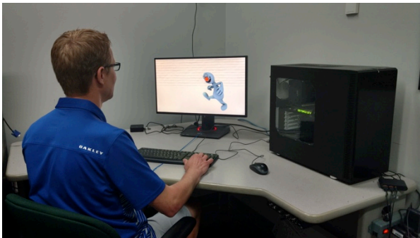
Fig. 1. Experimental setup, experiment taken in a dark surround with the participant at 2 picture heights away from the monitor
