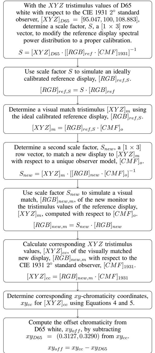
Fig. 6: Corresponding chromaticity simulation flowchart.
