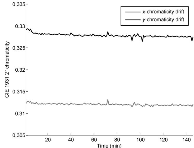
Fig. 12: Measured CRT phosphor chromaticity drift, 146 minutes.
