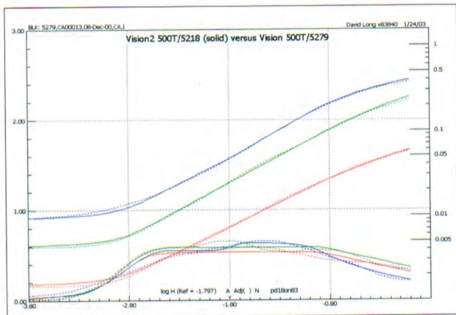
Figure 5. Sensitometry comparison of 5218 and 5279 films, with first derivative curves included to illustrate linearity.
