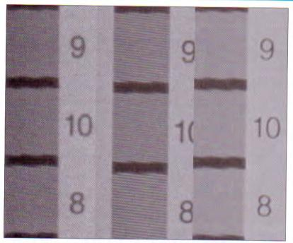
Figure 8. Enlarged view of portion of the ISO 12233 target—5218 Super 16mm (I) versus 35mm (c) and 24P (r).
