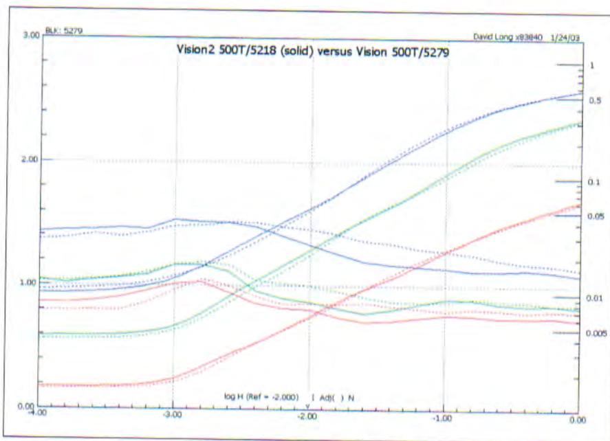
Figure 3. rms granularity comparison of 5218 and 5279 films.
