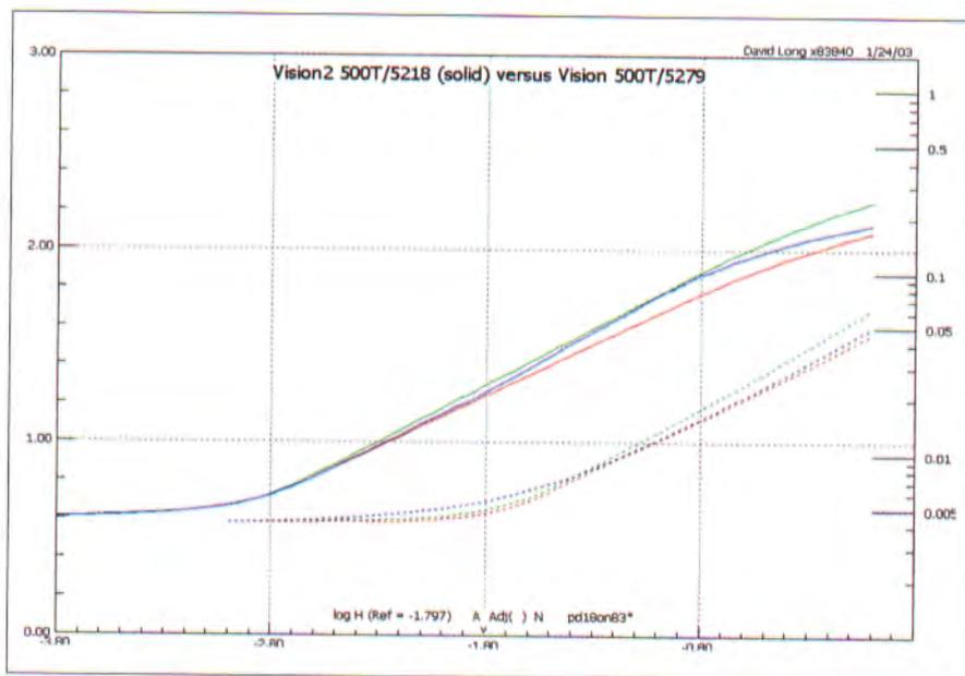
Figure 6. Toe sensitometry comparison of 5218 and 5279 films. Curves shifted vertically and horizontally to illustrate toe speed and sensitometry matches.
