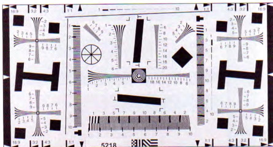
Figure 7. Low-resolution rendition of the ISO 12233 target.
