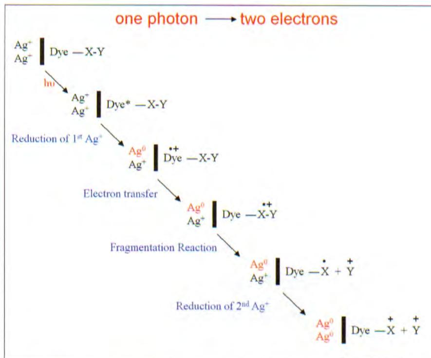
Figure 1. Illustration of the two-electron sensitizer mechanism.
