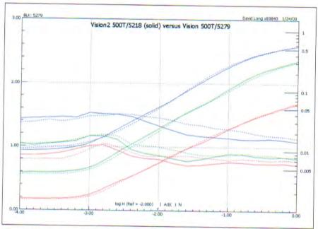
Figure 3. rms granularity comparison of 5218 and 5279 films.
