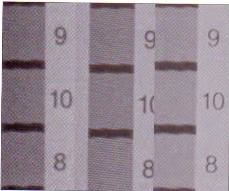
Figure 8. Enlarged view of portion of the ISO 12233 target—5218 Super 16mm (l) versus 35mm (c) and 24P (r).
