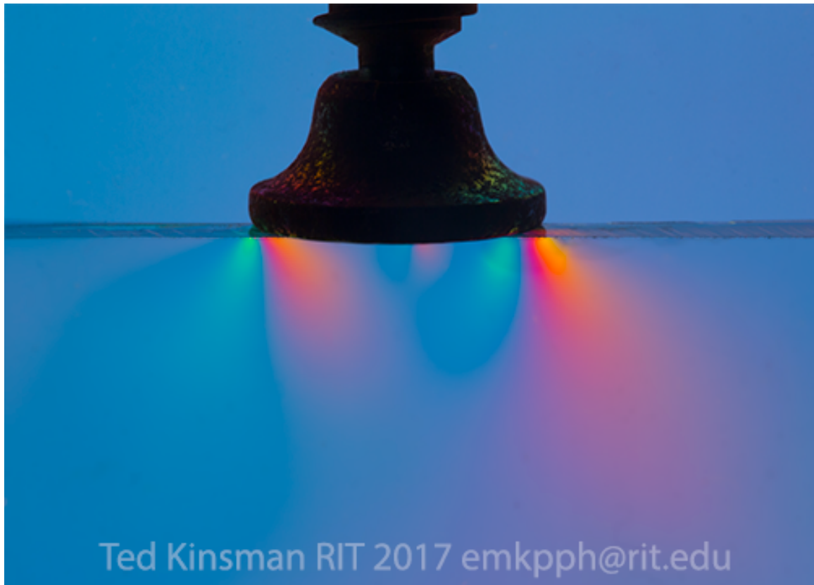
A close-up view of the stress created by a C-clamp with pressure applied to a block of glass.
