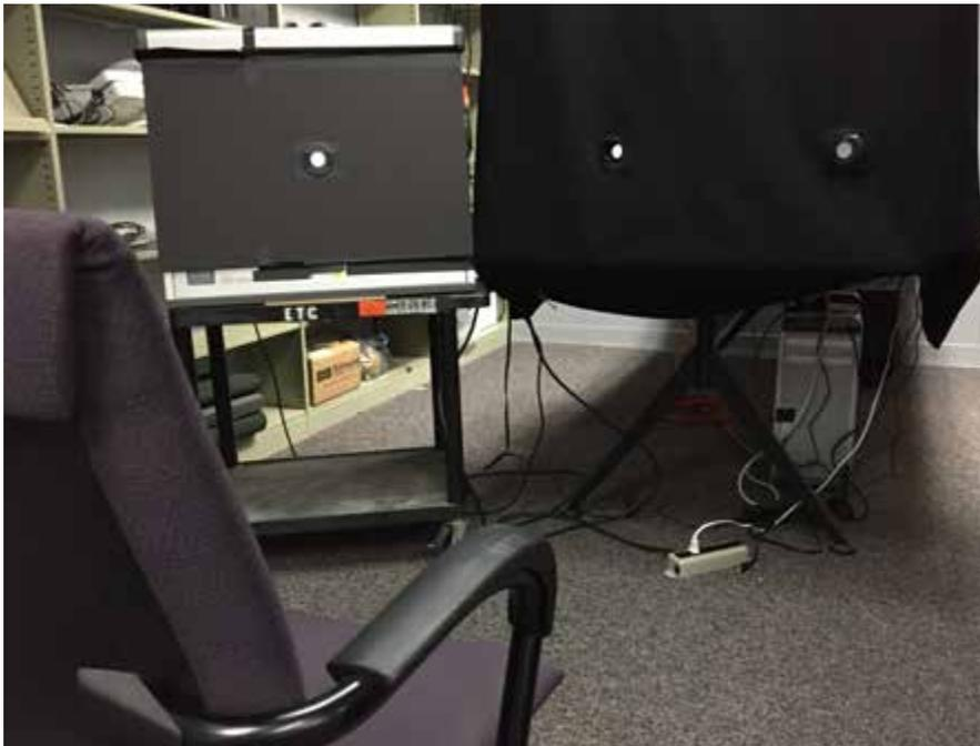
Figure 73. Two-alternative forced-choice experiment setup with aim stimuli produced using Color-aid papers in lightbooth on the left and reproduction systems presented through integrating sphere exit ports for two displays at a time on the right.
