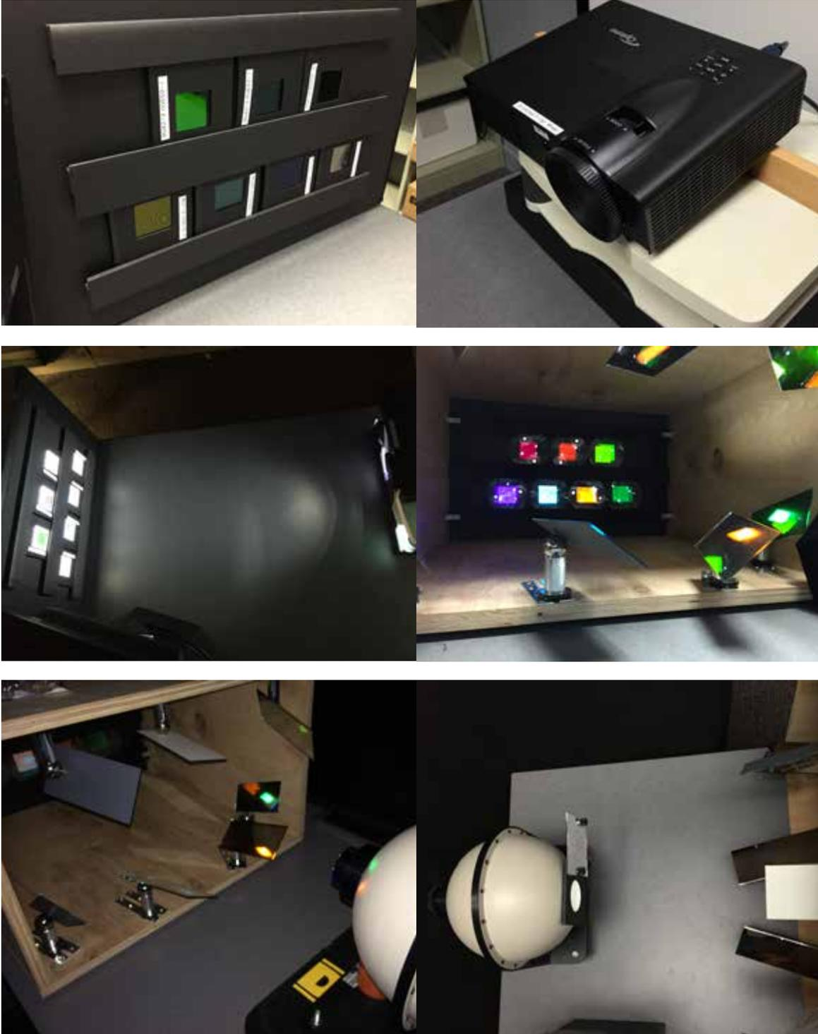
Figure 65. one-projector RIT MPD design images showing organization of seven-channel filters, monochromatic Optoma DX339 illumination source, focusing optics and integrating sphere for generating uniform spectral color stimuli for observer experiments
